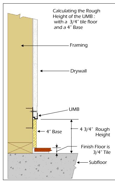
To continue our example, we have determined from the plans and a conversation with the architect that the base is to be 4" high.
